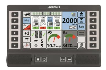
The iSOCAN Artemis system has the ability to work on ISOBUS ISO-compliant Universal Terminals, reducing the number of screens in the tractor cab.
